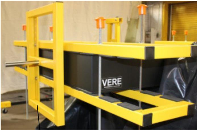
Mount the “Clamp Frames” to the table using the all-thread rods supplied and secured with nuts. These should only be tightened as much as hand tightening will allow. (4) rods will be used on each side as shown. Use the closest holes which allow the table to be balanced in respect to the center. Both sides of the table need to be done. **Place plastic caps on rods to prevent injury.**
