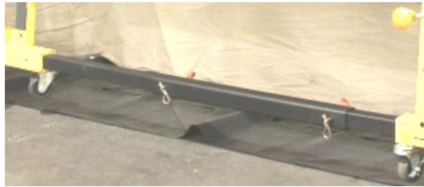
Select appropriate holes in “Connector Tube” and place “Hitch Pins” accordingly in each side.
