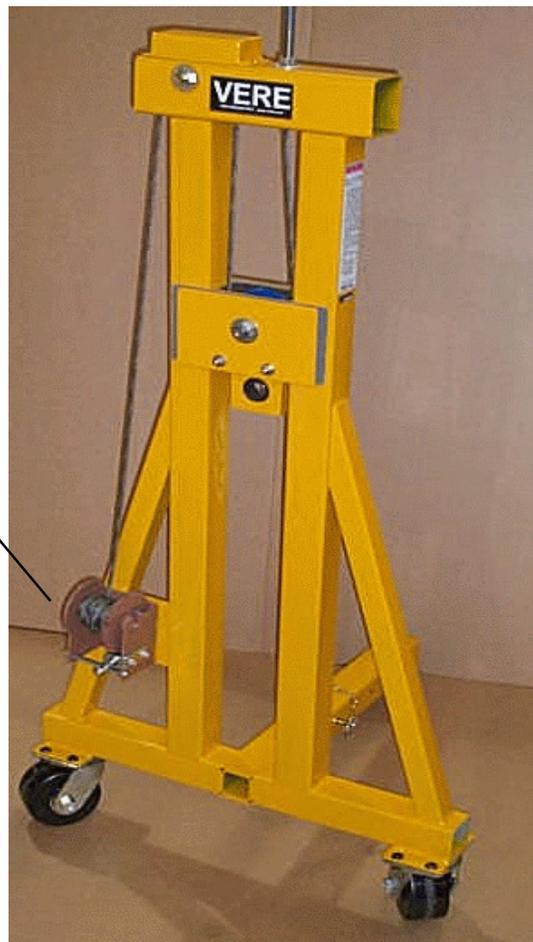
When raising the table, it is important that the table be raised uniformly. Both winches should be operated simultaneously. As the table is being raised, it may rotate suddenly. It is important that one person steady the rotation at all times.
